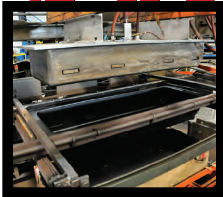
Pictured: Vacuum mold for keyboard case.
